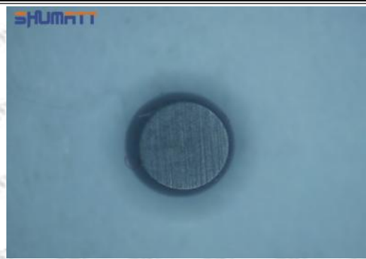
Semi ball's surface inspection
