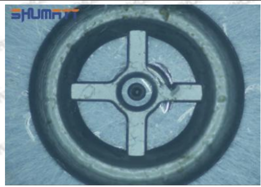
The misalignment of the semi ball causes damage to the orifice plate when installing it
