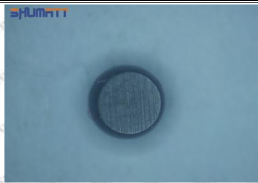
Semi ball's surface inspection
