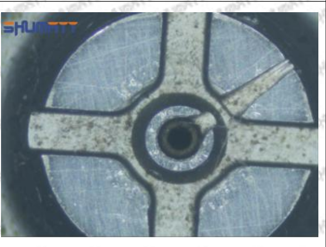
Washout marks caused by the presence of impurities in the fuel
